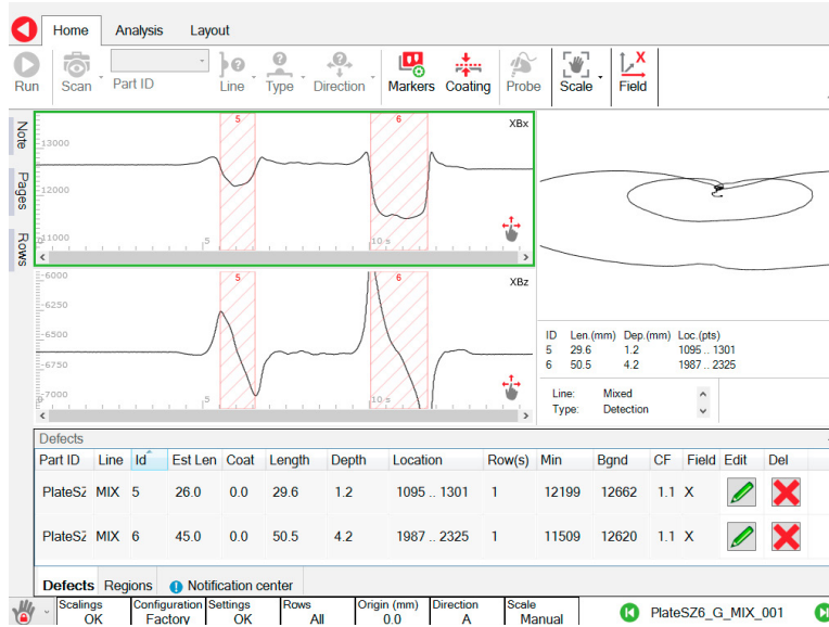
Figure 2-23 Defects dialogue box
