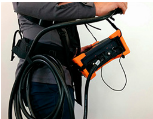
Figure 8-17 Belt-slinging probe cable
