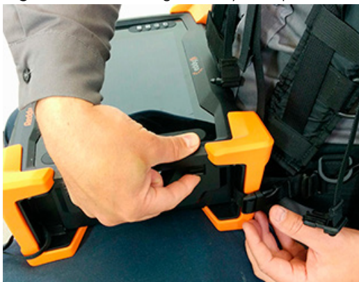
Figure 8-14 Closing battery compartment door.
